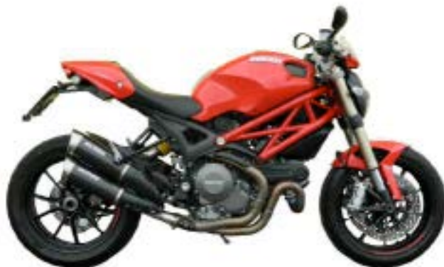
E3 GDU0828 _____ 5 9 EVO 5 Slip-on, STANDARD mounting with Y pi- pes and heat shield
